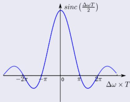
$$M[I] = 2q_{c/n_0} T \cdot \text{sinc}\left(\frac{\Delta\omega T}{2}\right) \rho(\Delta\tau) \cos(\Delta\omega T + \Delta\varphi)$$
